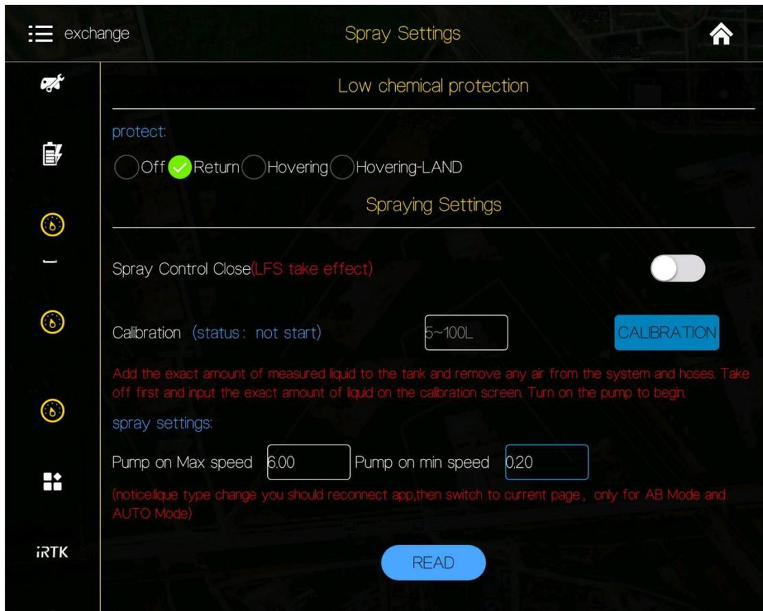
When liquid is nearly out, the following reaction could be set: Off(Close the protection), Return (auto home landing), Hovering, Hovering & landing. The default is Off, which means only LED flash as alarm. **We suggest you to set it on Return option.**
