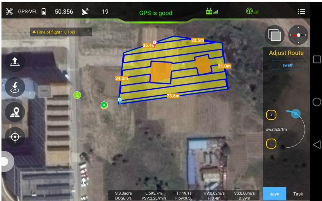
Swath(distance between 2 spraying route),obstacle gap(distance around the obstacle),target gap(distance between working area and boundary),offset(translation of working area).Save the task, then upload it by selecting block(working area).
