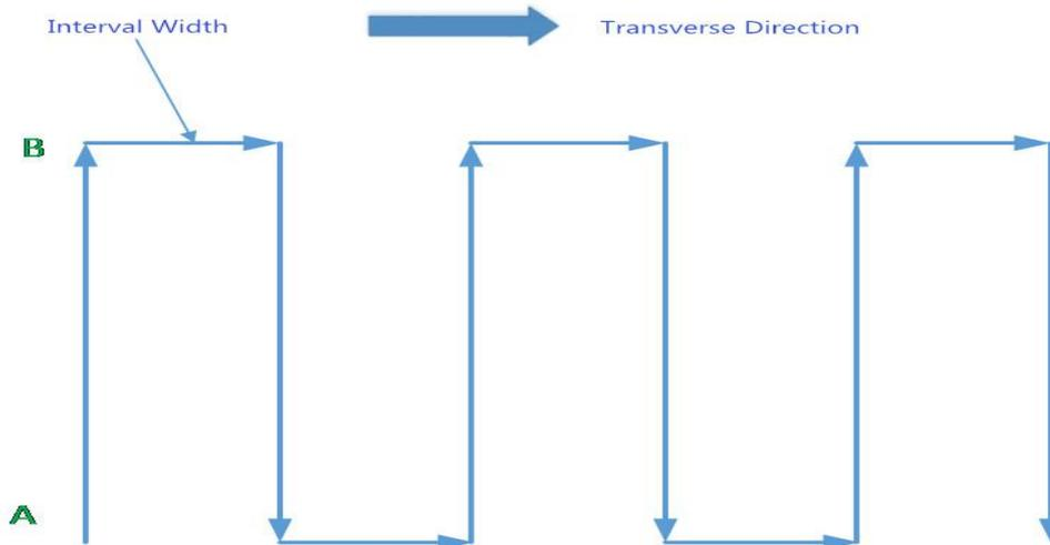
AB mode is a more simple efficient mode with fault tolerance to operate. The working theory is above in the picture. Record the point A and B, the UAV will plan the flight line like this.
