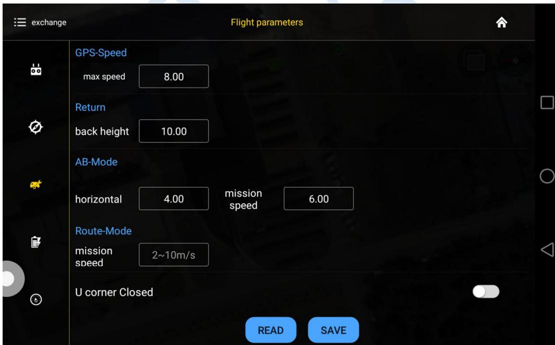
Click the button *READ* to obtain the current flying parameters,click button *SAVE* to save the parameters.
