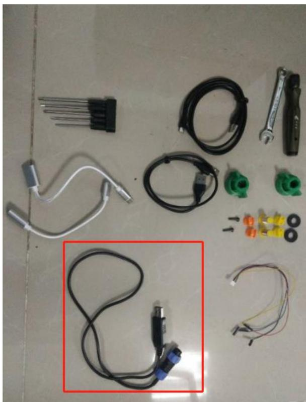
3 One connect to computer,another end connect to copter.Waiting for a moment(It takes few minutes to install the driver for the first connection with a new computer)
