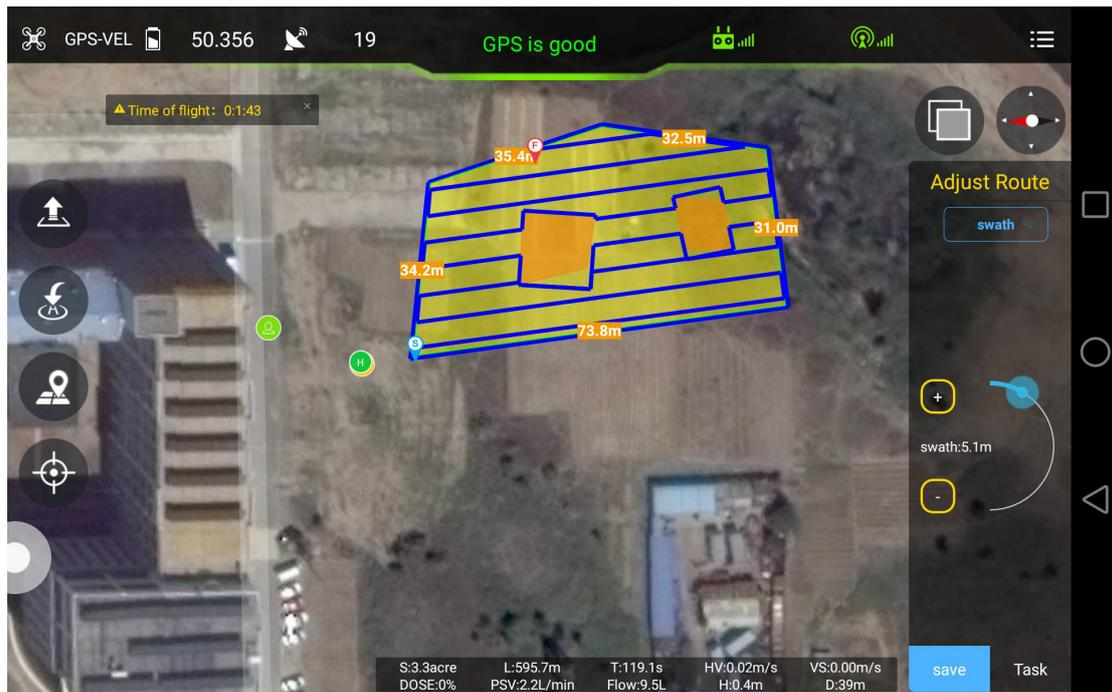
Swath(distance between each spraying),angle(angle of line),obstacle gap(distance around the obstacle),target gap(distance between working area and boundary),offset(offset of working area) in *Adjust Route interface*.Task could be saved according to demands,and then upload it by selecting block(working area).
